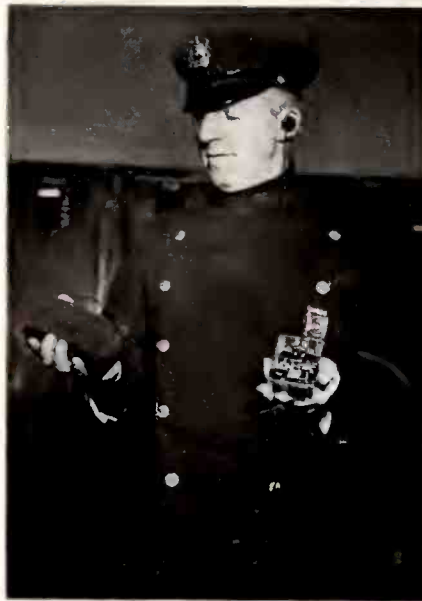
Pocket receiver employing bantam junior tubes, being used experimentally by Salem (Mass.) police.
