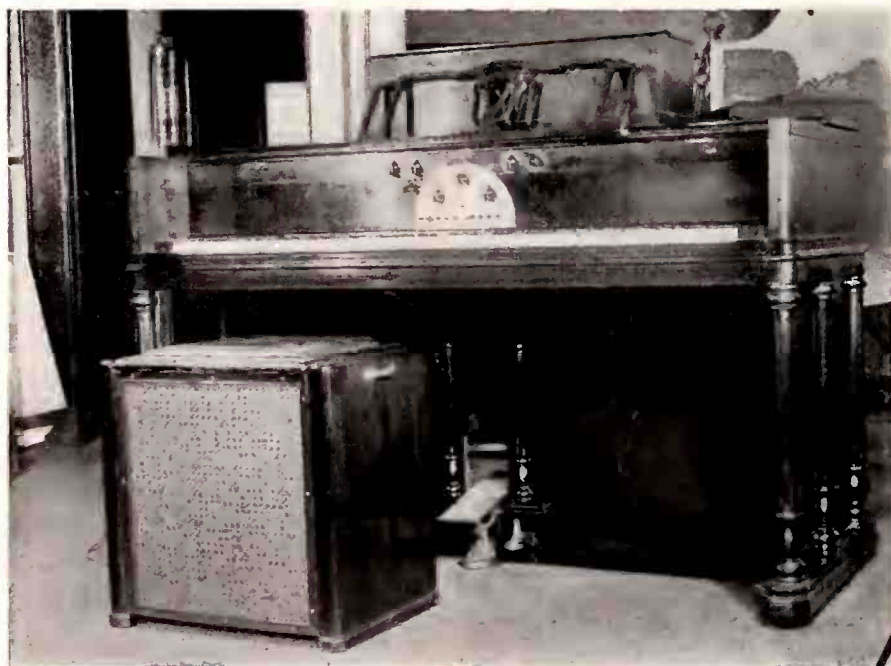
"Radio" piano developed by Miessner, using amplifiers and loudspeakers to provide great depth of tone and volume.
